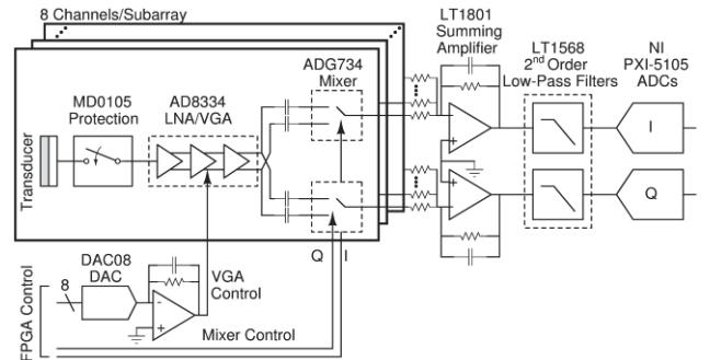
Figure 1: Subarray architecture for sub-Nyquist sampling AFE. 8 channels are beamformed using mixer-based beamforming and summed prior to digitization.
